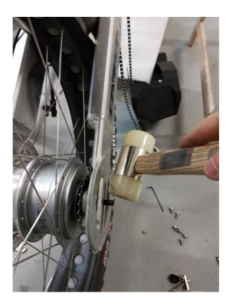
9) Check the presence of aluminum spacer in the back side of the brake caliper, especially before assembly the wheel
