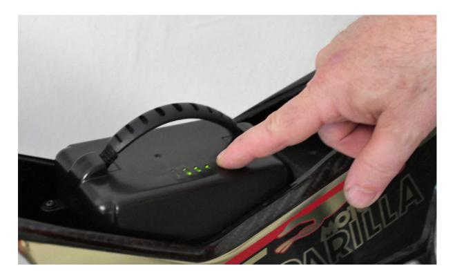
NOTICE: It is important that when the battery door is close the pin in the rear pasrt is well engaged in the carbon frame and that there are no wire on the top of battery case. All the wire must be stored on the back of battery case.
